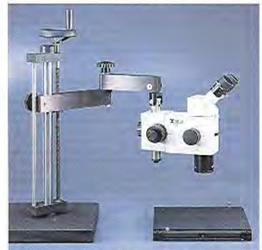
MA575 seen under RZ Stereo Microscope mounted on the MAC-3 Universal Stand
